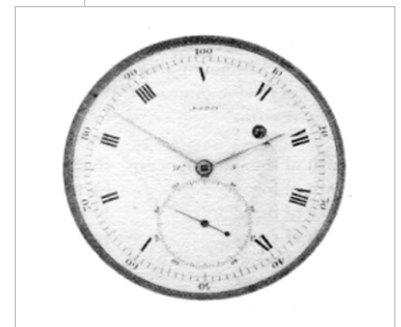
The 10 hour clock midday is 5 o'clock and midnight at 10 o'clock. - Musee des Arts et Metiers, Paris. Photo: Pascal Faligot
